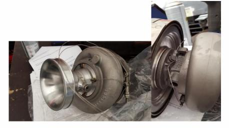
Examples of incorrect sealing wiring
